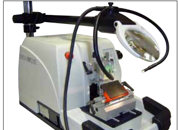
Fig 71, Leica rotary microtome with installed optional accessories: Magnifier and fiber-optic light guide
